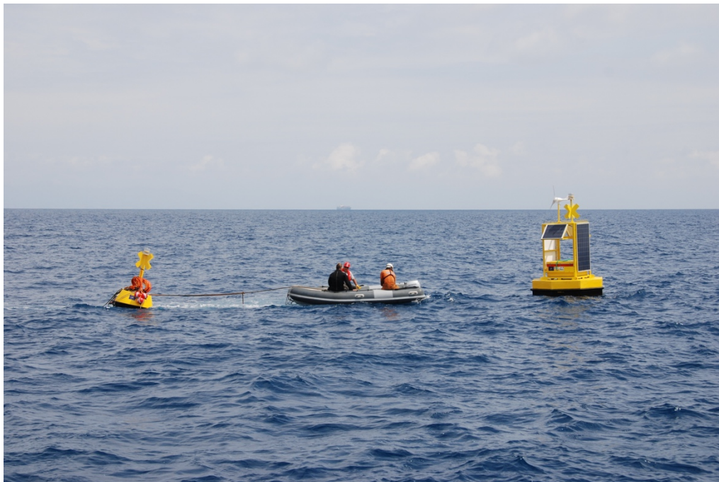
Figure 20: The operators link a secondary buoy with its primary
