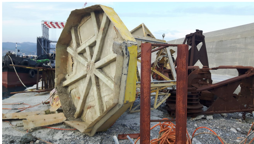
Figure 33: The upper part of the buoy from below. It lost completely all the buoyancy structure.
