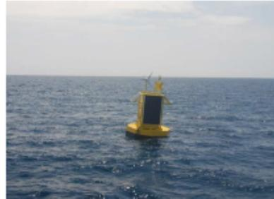
The detection unit is based on a main buoy (shown in the picture) equipped with solar panels and a data transmission system. Suspended to the buoy at a depth of 100 m, four hydrophones detect the cetaceans sound.
